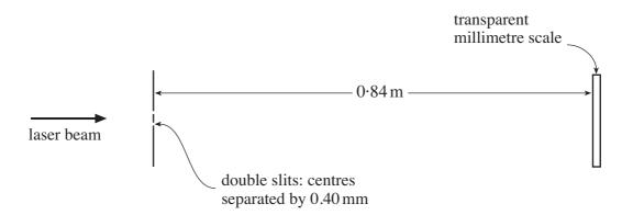
A transparent millimetre scale is placed 0.84 m from the double slits, as shown. When a camera is used to take a close-up picture of the scale, a series of equally-spaced bright and dark fringes is seen, as shown in the diagram below.
